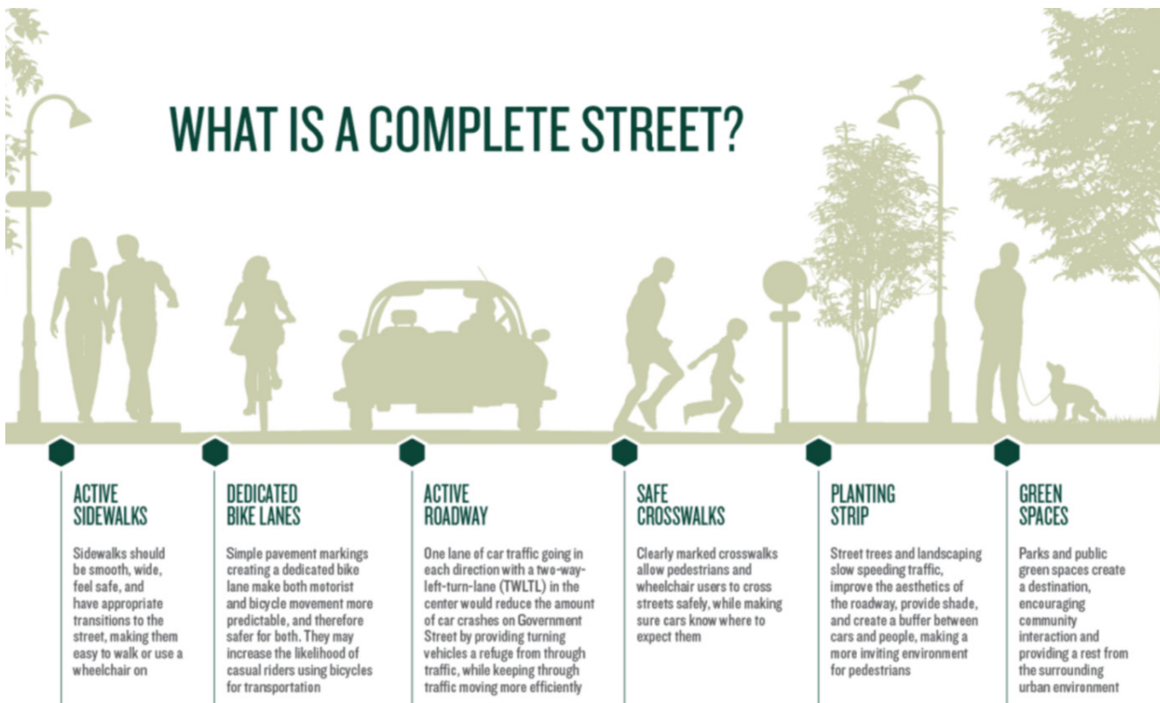
Figure 7.2: Complete Street Diagram
